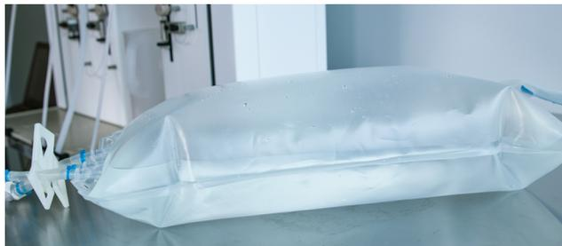
**Figure 15-8:** Swollen Bag When Using Open System
