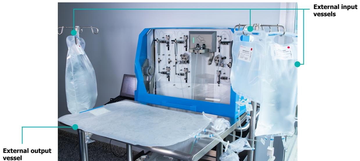
*Figure 15-5: Recommended Input Bag Layout*
