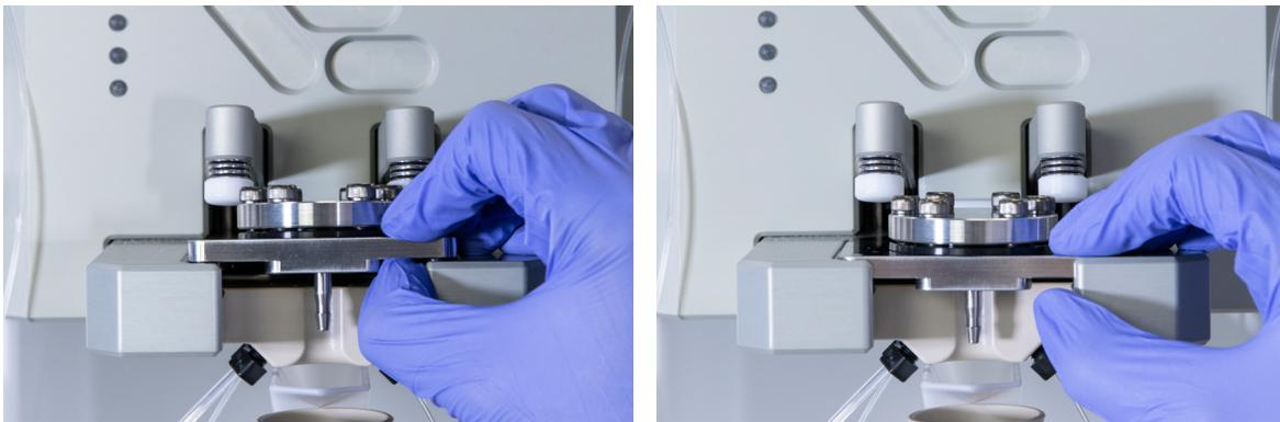
**Figure 8-1:** Installing a Blaze Cartridge
