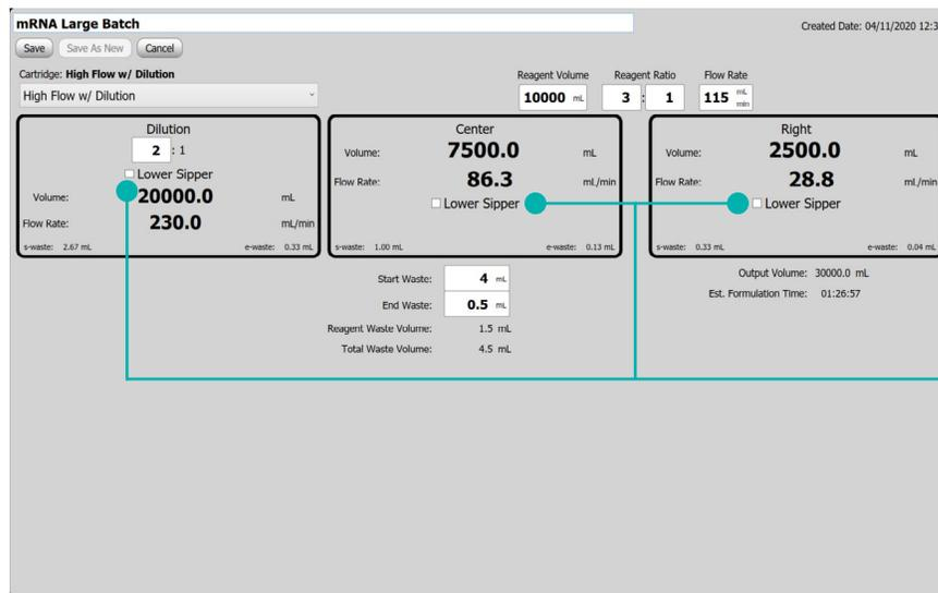
**Figure 15-3:** Recipe Tab with Lower Sippers Unchecked
