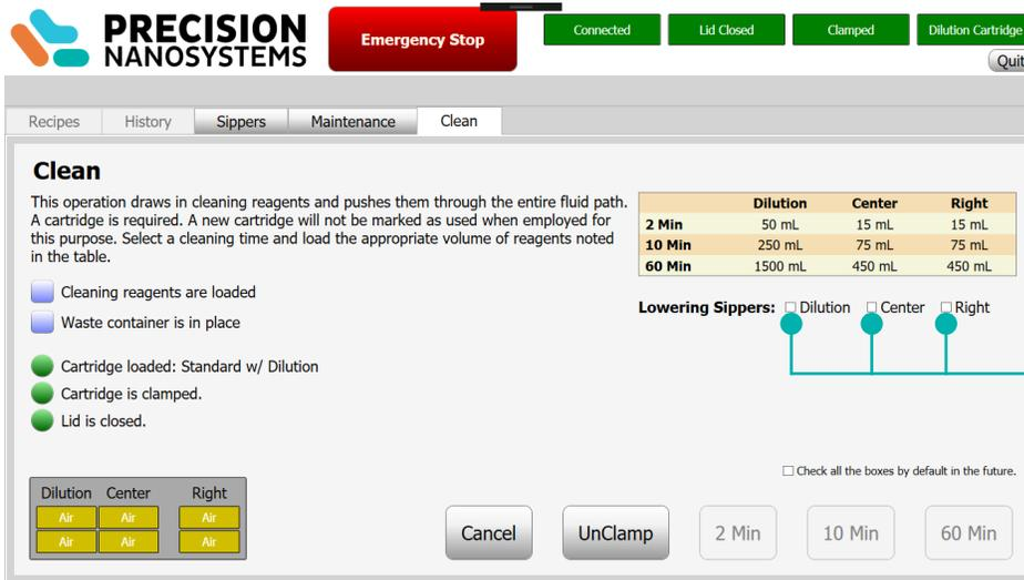
Figure 15-12: Clean Tab with Lowering Sippers Unchecked
