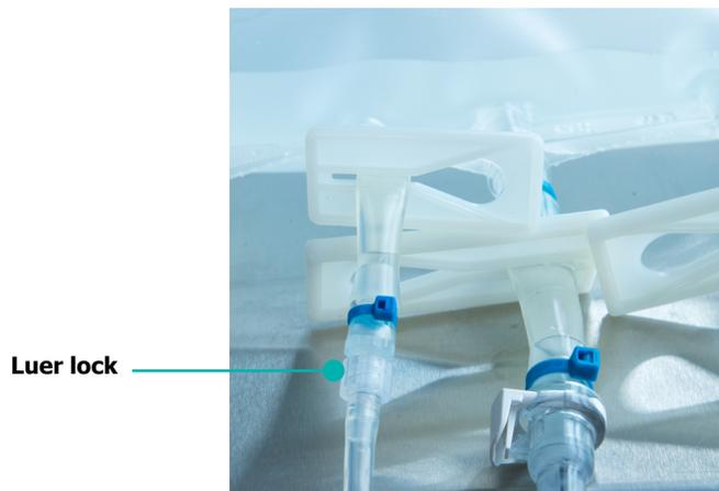
**Figure 15-6:** Bio-process Bag Connection and Valve
