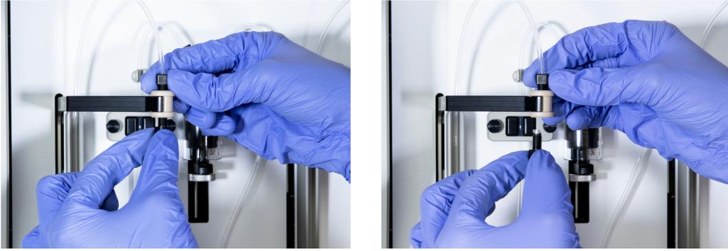
**Figure 13-3:** Replacing Sippers
