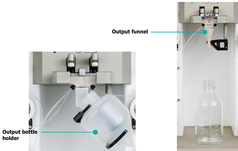
**Figure 8-5:** Output Vessel Arrangement
