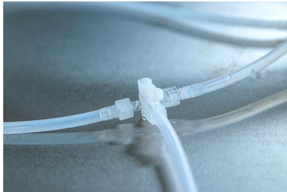
**Figure 15-10:** Closed System Tubing
