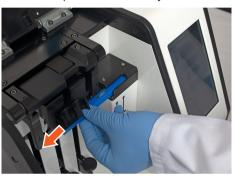
3 Hold the new sample arm with the tube holders on the left top side.
