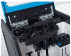
2 Insert the empty syringes selected for the run into the heating inserts in the R and C channels of the rotating block.
