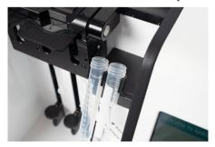
• If using the 100 mL sample arm on Ignite+: Make sure the lip of the waste tube is pressed upwards to sit as high as possible against the middle ridge of the tube holder. Make sure the lip of the 100 mL sample tube is pressed downwards to sit as low as possible on the top edge of the tube holder.
