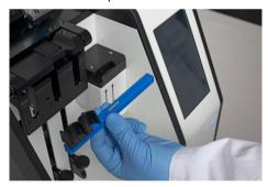
4 Align the body of the sample arm with the holder on the instrument.
