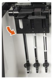
7 Install the sample collection tube in the right clip of the sample arm and the waste collection tube in the left clip of the sample arm.
