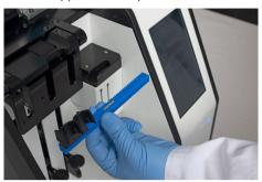
5 Align the body of the sample arm with the holder on the instrument.
