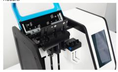
Insert the R, C, and optional L syringes into the respective channels of the rotating block.
