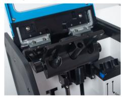
If using Ignite+ heating inserts, the three arrows on the insert must point in the direction of the fluid flow.
