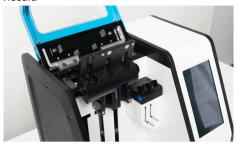
3 Insert the heating insert or inserts into the appropriate channel of the rotating block.
