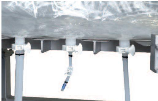
6. Close all clamps on the outlet lines and ensure that the inlet lines are open on the biocontainer. Secure the lower swivel door and replace locking pin. Attach the four hoist clips to the holes four holes located at each corner of the top of the biocontainer. Ensure each clip fastens to the corresponding hole so that the crossbar is holding the four connection points (Figure 22).
