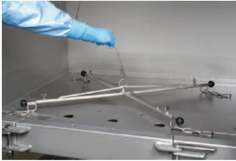
7. To extend the cross frame arms, turn the knob on each arm and slide each arm to the four tote corners. The cross frame arms should be adjusted so they are 15 – 20 mm from the tote inner corners (Figure 16).
