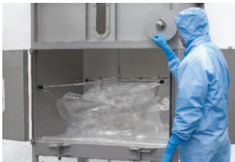
3. The Allegro biocontainer should be raised so that the crossbar with the Allegro biocontainer connected is near the top of the extension module (Figure 24).
