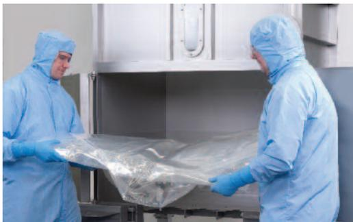
**Note:** Two operators are recommended to perform Allegro biocontainer installation
