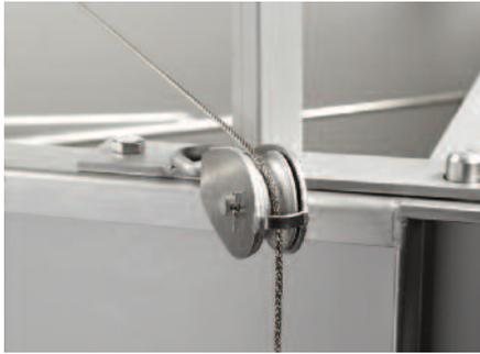
3. Slide the other end of the stainless cable through the small hole located inside the friction wheel. Connect the cable lock to the cable by sliding it over the cable and fastening the two flat head screws secure it to the cable. This will prevent the cable from disconnecting from the friction wheel. (Figure 13)
