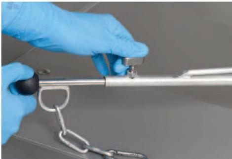
8. Using the friction wheel, raise the crossbar inside the tote to prepare for biocontainer installation (Figure 17).
