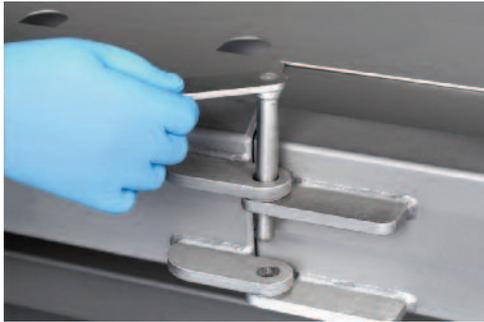
10. The swivel locking plate is used to secure and unsecure the ports of the Allegro biocontainer and needs to be opened to install the Allegro biocontainer. (Figure 19).
