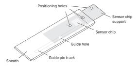
The sensor chip is fixed to a polystyrene sensor chip support. Each cassette, consisting of a sensor chip and sheath assembly, is packed in a separate pouch and sealed under a nitrogen atmosphere.
