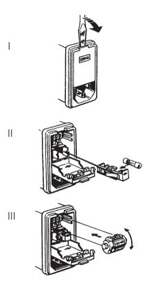
4 Place the fuse appropriate to your mains supply voltage in the fuse holder and insert it into the right-hand position (step II in the illustration). The left hand position is a holder for a spare fuse (included in the Mains Kit).
