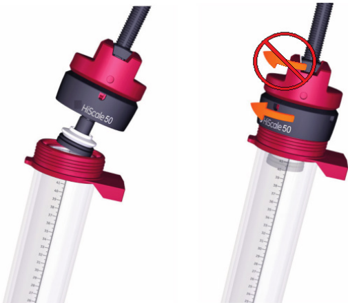
Fig 8. Inserting and fastening the adapter into the column tube, steps 5-6. Step 6 Fasten the adapter to the column tube by turning the end housing down. Holding the end cap still while doing so keeps the shaft and plunger from spinning.
