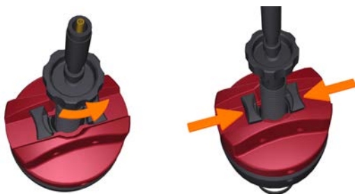
Fig 11. Adjusting the adapter position using QuickLock, steps 4-5.
