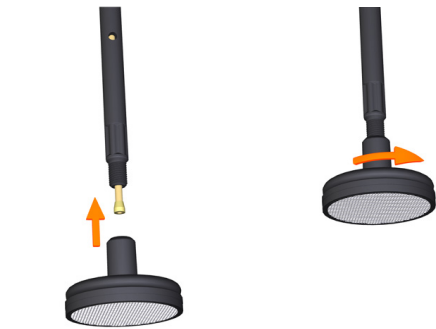
Fig 4. Replacing the capillary tubing, steps 2-4.
