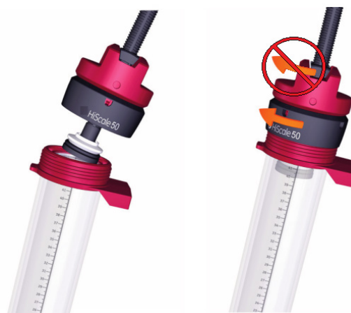
Fig 8. Inserting and fastening the adapter into the column tube, steps 5-6. Step 6 Fasten the adapter to the column tube by turning the end housing down. Holding the end cap still while doing so keeps the shaft and plunger from spinning.
