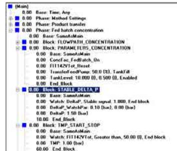
The list in the **Text Instructions** tab has a tree structure and individual blocks can be expanded or contracted, as indicated by the **+** or **-** signs. When expanded, all the block instructions and nested blocks are displayed and available for editing.
