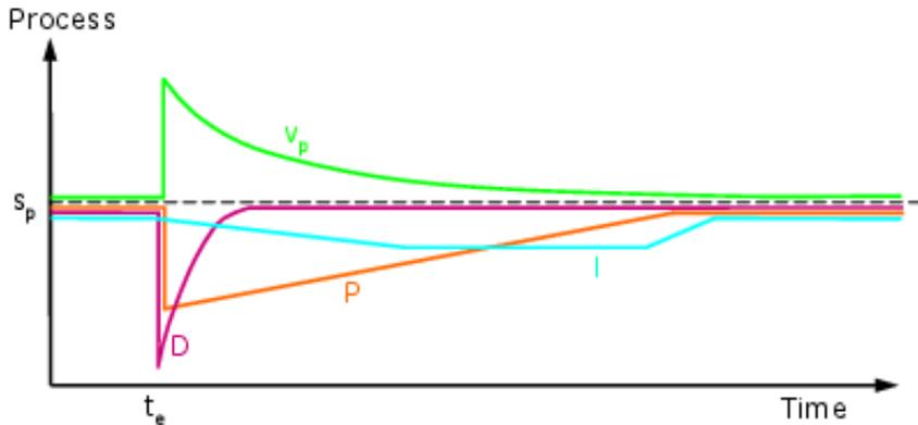
This illustration shows the behaviour of the P, I and D components of a typical PID process control regulator.
