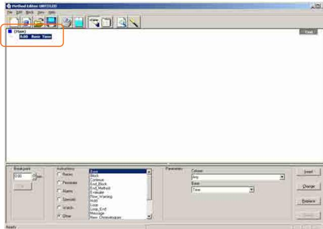
The new method will be displayed in the **Text** pane as the **Main** block with a single **Base Time** instruction.
