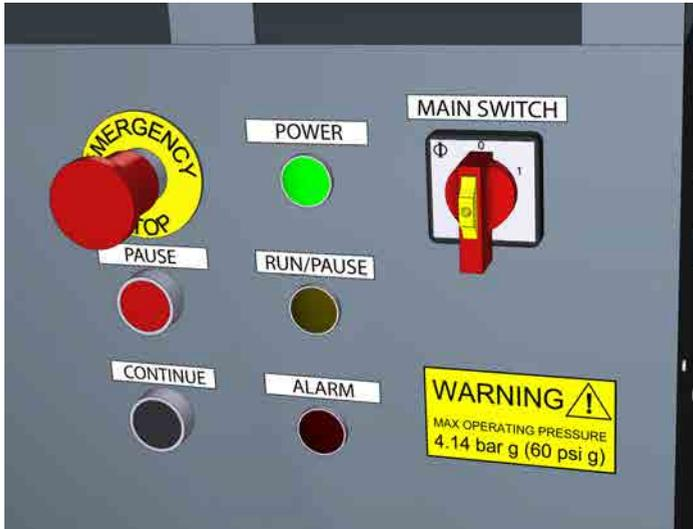
**Note:** The **EMERGENCY STOP** and **MAIN SWITCH** controls are not part of UNICORN and are described in [Section 2.3 Emergency procedures, on page 25](#).
