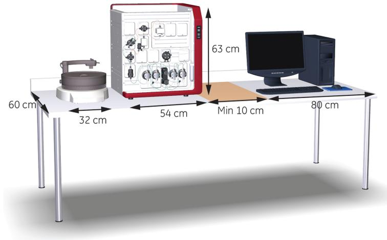
The illustration below shows the space recommended for ÄKTA pure with Fraction collector F9-C.
