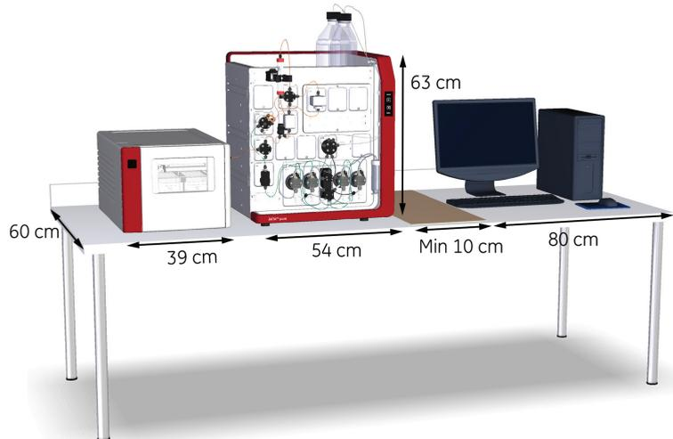
**Note:** There must be at least 10 cm free space on the right side and behind the ÄKTA pure instrument, to allow for adequate ventilation.
