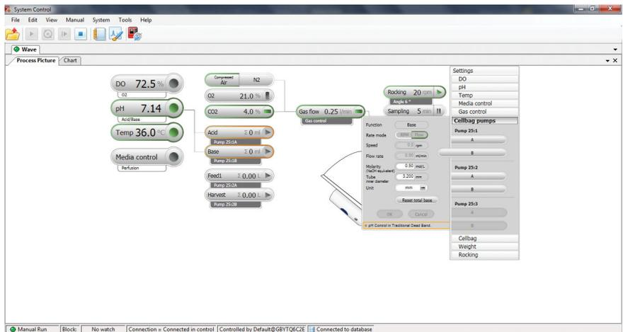
The following example shows the **Process Picture** display when the system is in CO<sub>2</sub> deadband mode.
