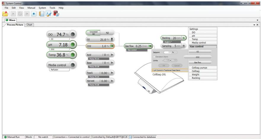
The following example shows the **Process Picture** display when the system is in CO<sub>2</sub>/Base deadband mode.
