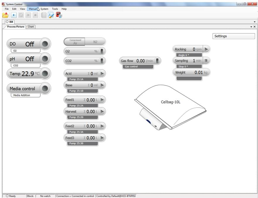
Items in the process picture reflect the components included in the system (for example, the illustration above shows a system in single mode equipped with three pumps).
