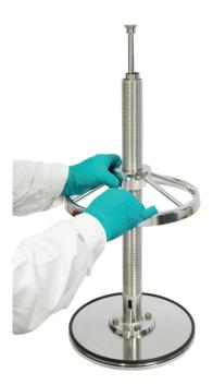
7 In a counter clockwise direction, screw down the top plate assembly 5 cm along the outer adapter tube.
