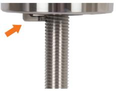
For 300 and 450 columns only: Remove the stop screw and locking nut from the adapter top plate.
