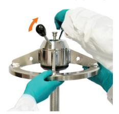
7 Unscrew the bolts on the upper ring of the sealing unit. This will release the sealing unit and the inner adapter tube.
