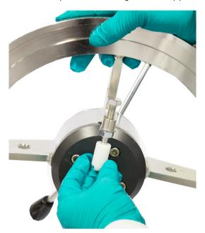
Put the spring inside the plastic end socket and assemble them together with the stop screw and locking nut on the top plate.
