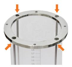
6 Align the inner surface of the glass tube with the inner surface of the flange.
