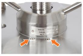
3 For 200 columns and smaller sizes: Remove the stopper.
