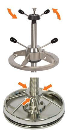
Use a flashlight and a screwdriver through one hole to adjust the inner tube in position. Add two adapter head screws but do not tighten them.
