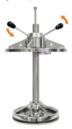
8 Assemble the seal adjuster on top of the adapter.
