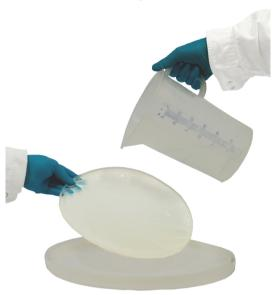
Wet the net with 20% ethanol to remove all air bubbles trapped in the net. If the net is tight when refitting, warm it in 50°C water to soften it and to get it in place easier.
