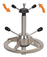
6 Remove the top-plate assembly by turning it in a clockwise direction.
