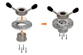
3 Slide the spring (c), inner adapter tube (b) and outer adapter tube (a) onto the adapter plate.
