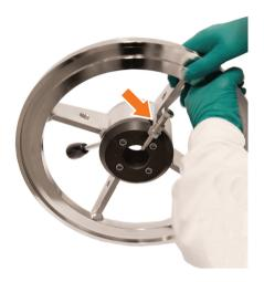
5 Carefully unscrew and remove the seal adjuster. This releases the tension on the spring situated under the inner adapter tube.
