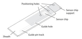
The sensor chip is fixed to a polystyrene support sheath. Each cassette, consisting of a sensor chip and sheath assembly, is individually packed under a nitrogen atmosphere in a sealed pouch.
