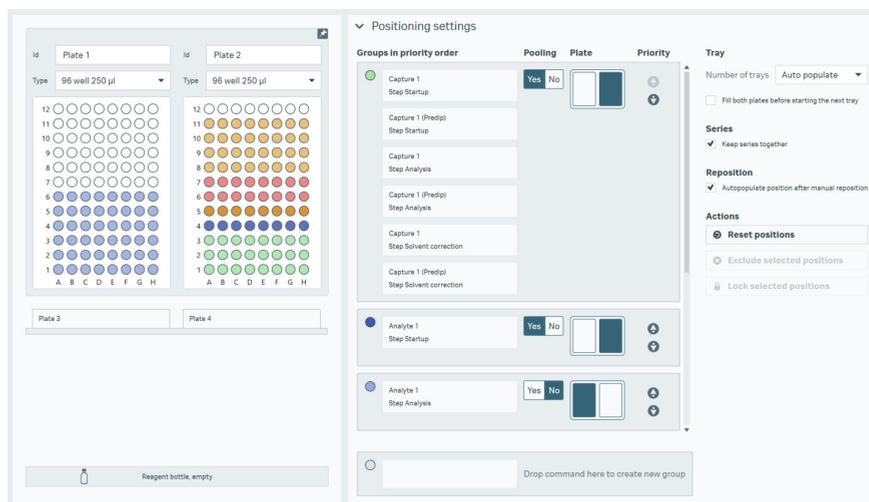
Solutions may be grouped together so that the settings apply to all solutions in the group. To split a group, drag one of the commands from a group to the empty placeholder at the bottom of the group list. To combine solutions in a group, drag the solutions together. The following settings apply separately to groups:
