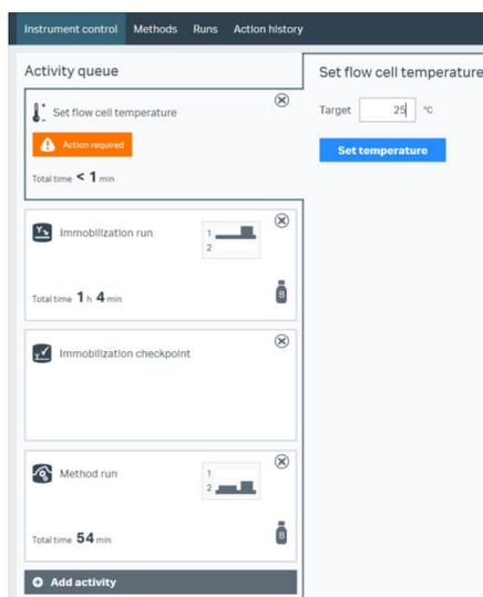
An activity that is added to the queue will start automatically when required user input has been provided and all previously queued activities are completed. Conditions that prevent a run from starting are highlighted in orange.
