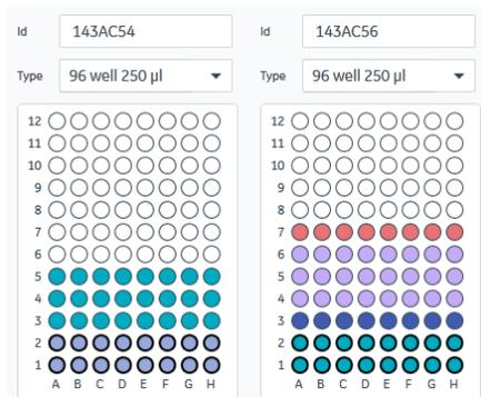
**Note:** You may use a barcode reader to enter the microplate **Id** if you are using coded microplates. The microplate **Type** is not however linked to the microplate barcode. Make sure that the correct **Type** is selected.
