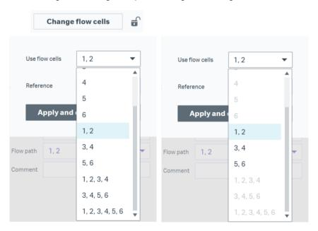
The **Reference** setting of analysis methods is automatically adjusted based on flow cell selection and cannot be changed upon procedure start. For Biacore 8 series, the flow cell selection of a procedure is always locked.
