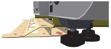
5 If a rotation guide is used, attach the second bolt in the rotation guide.
