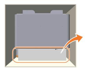
9 Use a flat screwdriver to lever up the fastening tabs on the sides. Start in one corner, then continue to the diagonal corner, then the remaining two corners.
