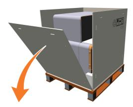
Lift the bottom of the crate side straight up, thus unhooking the bottom from the pallet.
