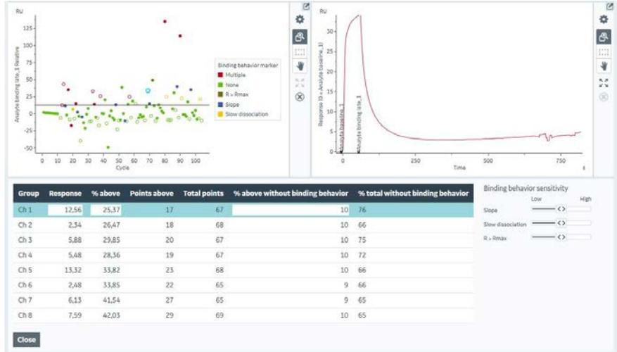
The function also analyses the sensorgrams to identify atypical binding behavior that is relatively common in fragment screening work. The plot points are colored by binding behavior indicators when **Binding level screen cut-off** is applied. The following atypical binding may be identified:
