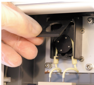
Figure 5.3: Closing the cover of the peristaltic pump.
